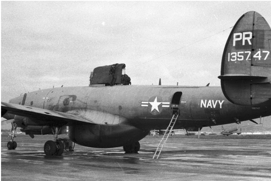
PR-24 AT TAIPEI, TAIWAN, 4 JANUARY 1961 AFTER LOSING UPPER RADOME DIVING AWAY FROM CHICOM FIGHTERS
